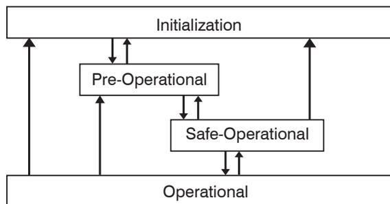
Abb. 87 EtherCAT State Machine
