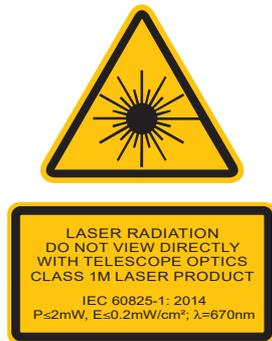
Fig. 1 Laser warning sign and laser label
