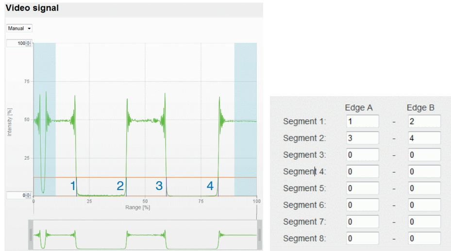
Fig. 35 Video signal with defined segments
