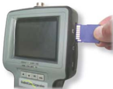
Fig. 4 Installing the SD Memory Card
