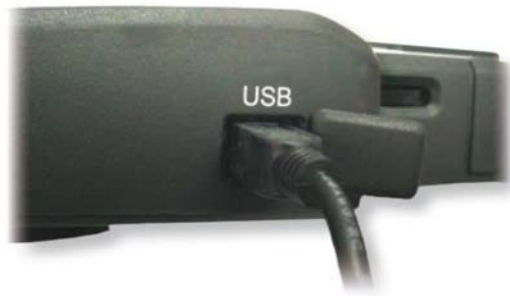
Fig. 10 Connection USB cable to video endoscope
