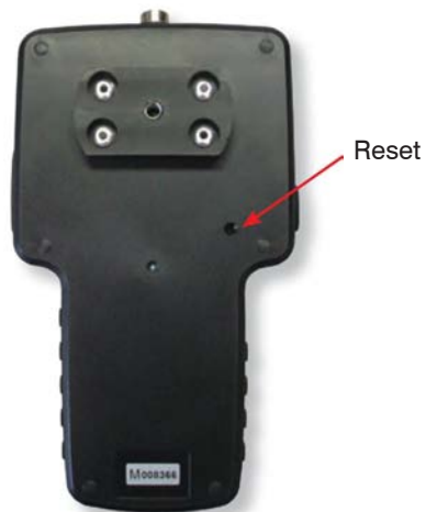
Fig. 11 Back side of the video monitor with reset button
