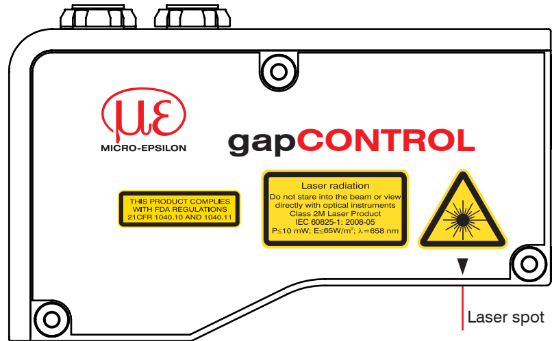
Fig. 1 True reproduction of the sensor with its actual location of the warning label
