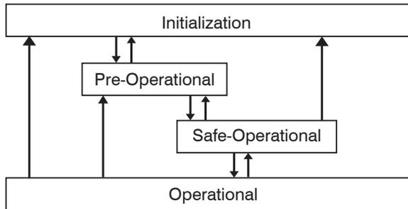
Fig. 66 EtherCAT State Machine
