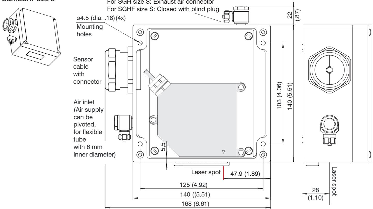
Fig. 61 Protective housing for measuring ranges 2/10/20/50/100 mm
