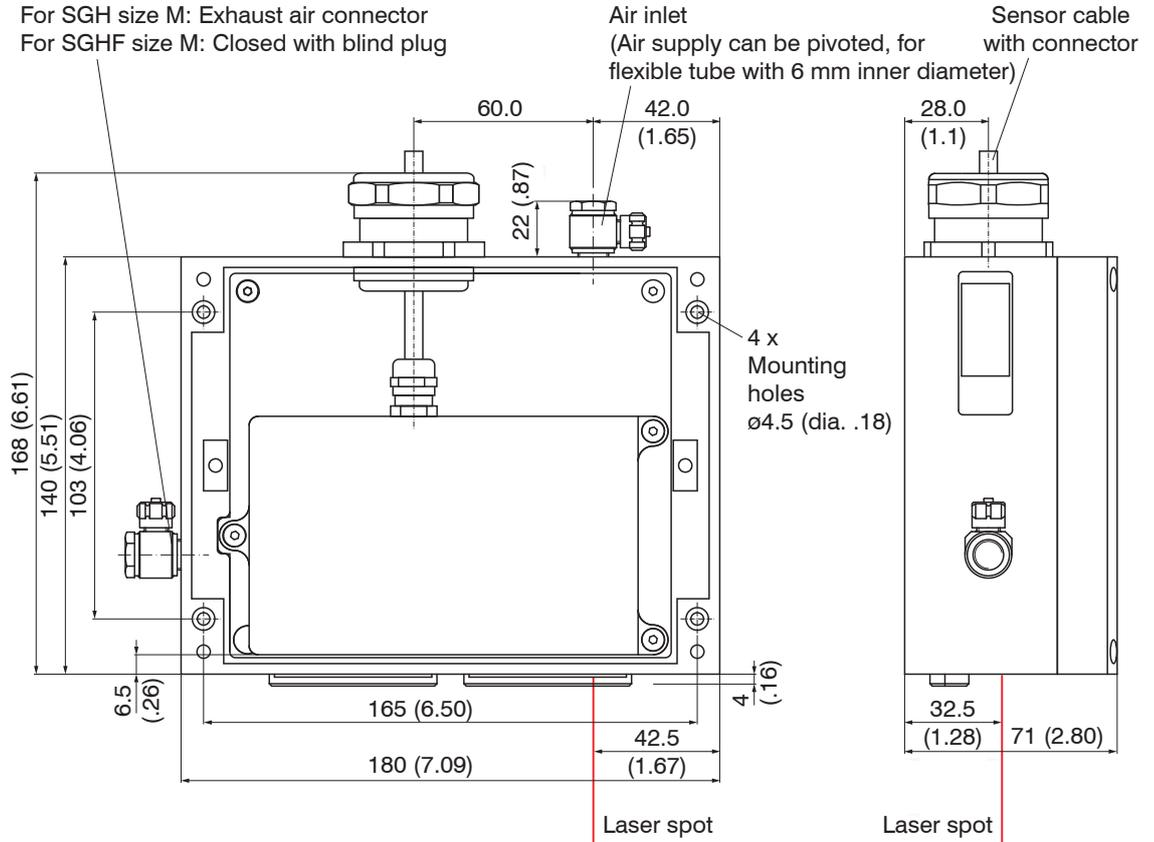
Fig. 62 Protective housing for measuring range 40 and 200 mm
