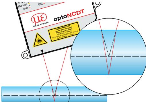
For measurements on transparent targets, such as films, it is due to the refractive index to smaller measurement values than it is actually the case.
