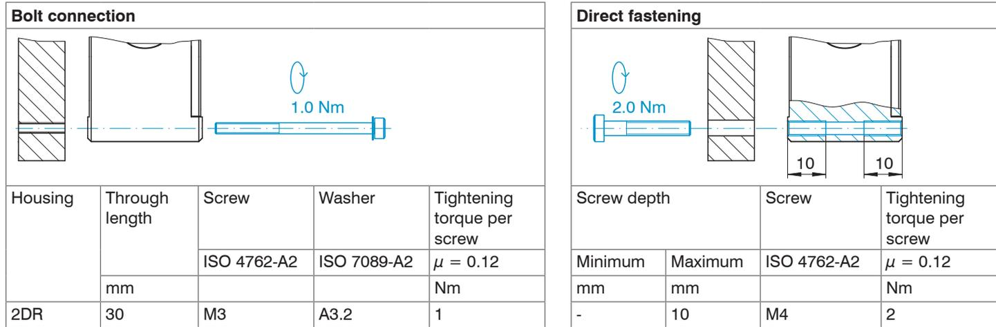
Fig. 18 Mounting conditions housing size 2DR
