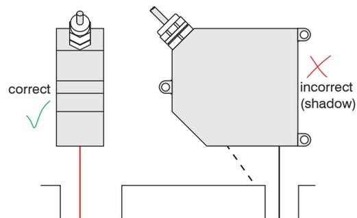
In case of bore holes, blind holes, and edges in the surface of moving targets the sensor must be arranged in such a way that the edges do not obscure the laser spot.
