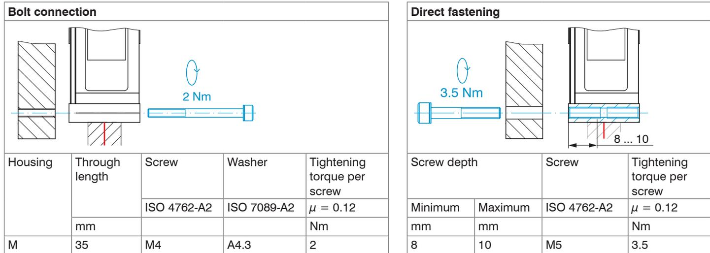
Fig. 13 Mounting conditions housing size M
