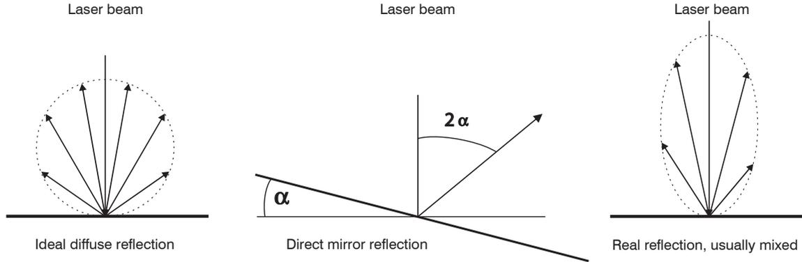
*Fig. 56 Reflection factor of the target surface*
