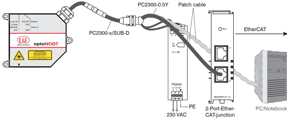
Fig. 26 Measurement setup with EtherCAT connection
