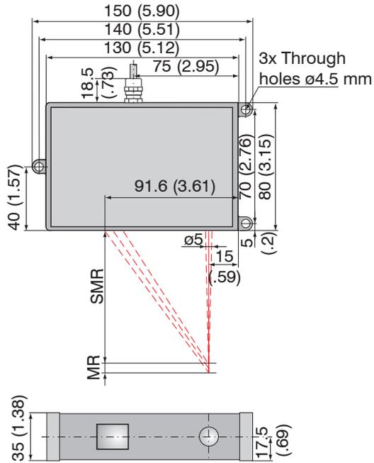
Fig. 15 Dimensional drawing ILD2310, measuring ranges 10/20/40 mm
