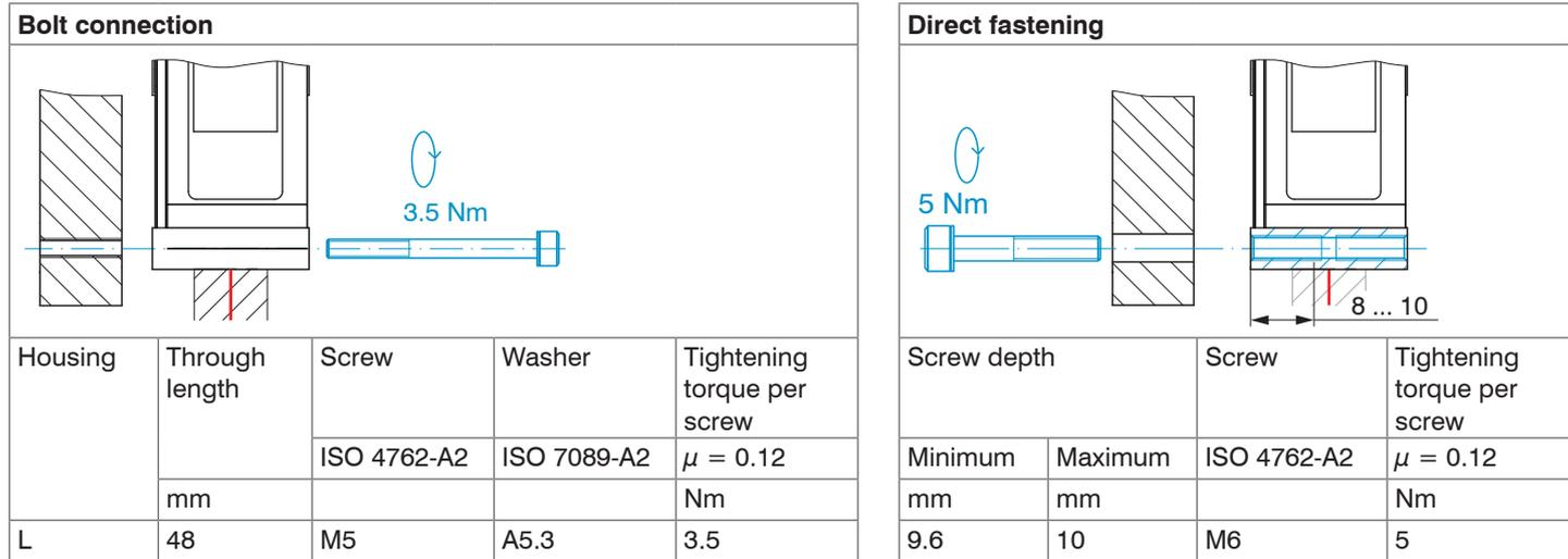
Fig. 16 Mounting conditions housing size L
