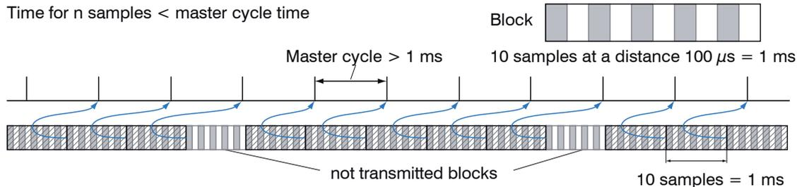
If the number of samples selected is too high, i.e. the time for the filling of a block is longer than the master cycle time, each block is picked up by a master cycle. However, single blocks and therefore samples are transmitted twice or even more often. This can be detected on the master side by the transmission of the Timestamp or Valuecounter, see object 0x21B0.
