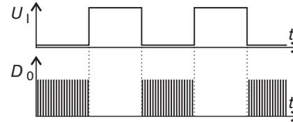
Fig. 40 Low trigger level (above) and digital output signal (below)
