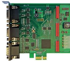
The IF2008/PCIE interface card enables the synchronous capture of 4 digital sensor signals series optoNCDT 2300 or others or 2 encoders. In combination with IF2008E a total of 6 digital signals, 2 encoder, 2 analog signals and 8 I/O signals can be acquired synchronously.
