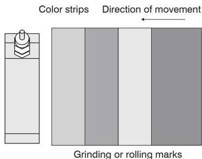
In case of rolled or polished metals that are moved past the sensor the sensor plane must be arranged in the direction of the rolling or grinding marks. The same arrangement must be used for color strips.
