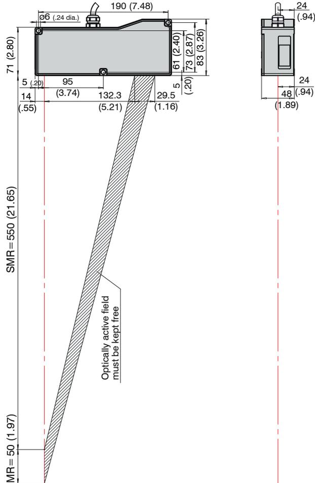
Fig. 17 Dimensional drawing and free space for the sensor ILD 2310-50
