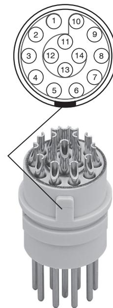
Fig. 24 Sensor round pin plug, view: Solder-pin side male cable connector, insulator
