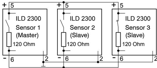
The signals Sync-in/out or /Sync-in/ of same polarity are connected in parallel with each other. A sensor is to program as a synchronous master, which supplies the subsequent slave sensors with symmetric synchronous pulses, RS422-level. Only in the last slave sensor in the chain the terminating resistor is activated of 120 Ohm, see Chap. 7.6.3. The system grounds (pin 2) of the sensors are to connect to each other.
