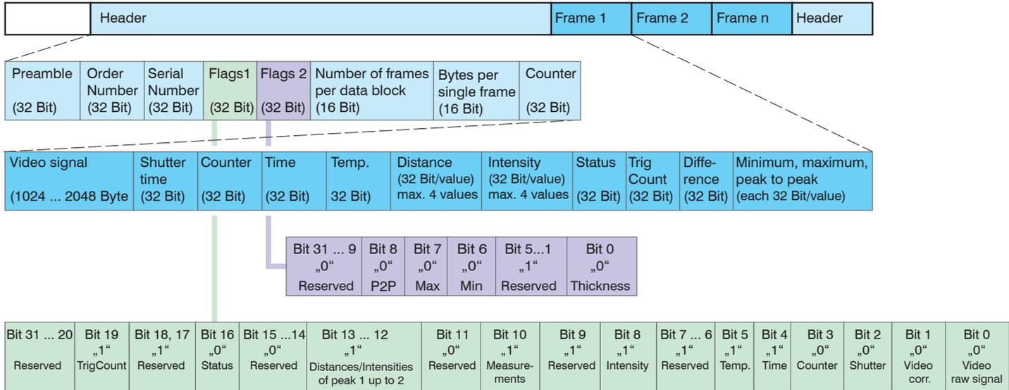
Fig. 69 Example for a data transmission with Ethernet
