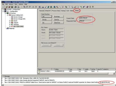
To configure the synchronous manager correctly, it is first necessary to read the object directory of IL2300:
