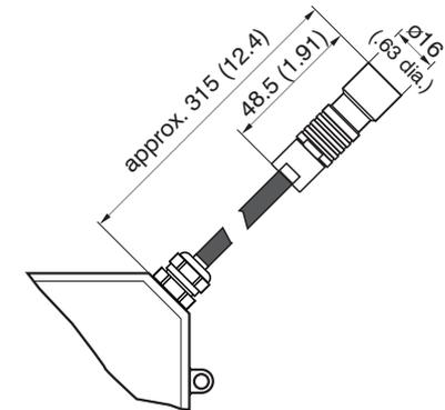
Fig. 9 Dimensional drawing sensor cable
