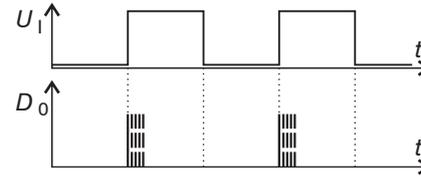
Fig. 41 Trigger edge LH (above) and digital output signal
