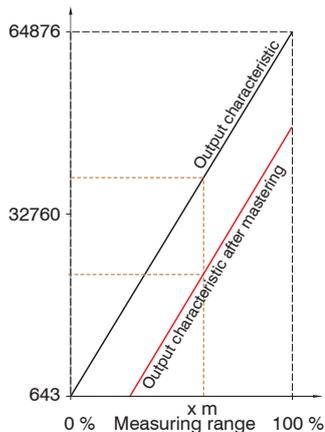
When mastering the sensor’s characteristic is parallel displaced. The displacement of the characteristic curve reduces the usable measurement range of the sensor the further the master value is away from the master position.
