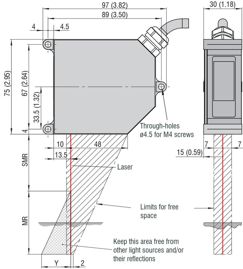
Fig. 11 Dimensional drawing, free space for diffuse reflection
