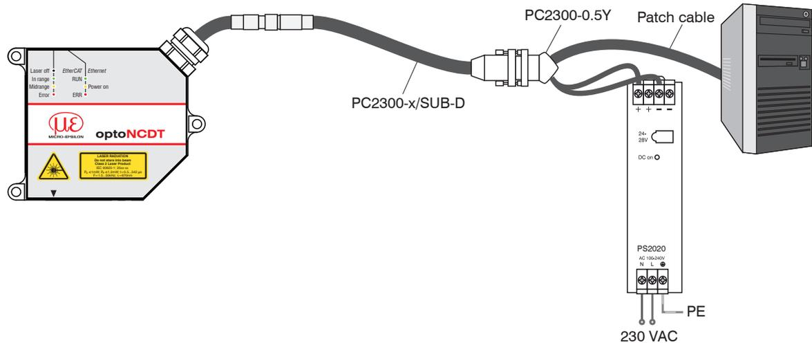
Fig. 25 Measurement setup with Ethernet connection
