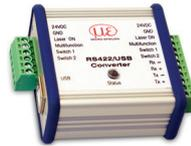
Converter RS422 to USB, type IF2001/USB, useable for cable PC2300-X/OE or PC2300-X/SUB-D + PC2300-0,5Y, inclusive driver, connections: 1 x female connector 10-pin (cable clamp) type Würth 691361100010, 1x female connector 6-pin (cable clamp) type Würth 691361100006
