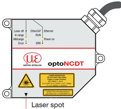
Fig. 1 Sensor with its actual location of the warning labels, ILD2300
