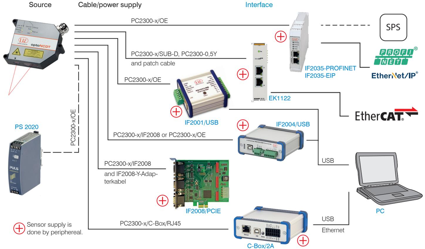
Fig. 20 Connection examples on ILD2300 optoNCDT 2300
