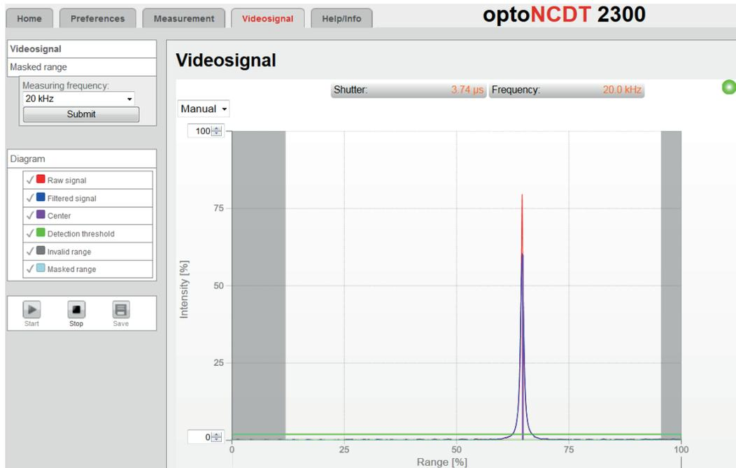
Fig. 30 Display of video signals
