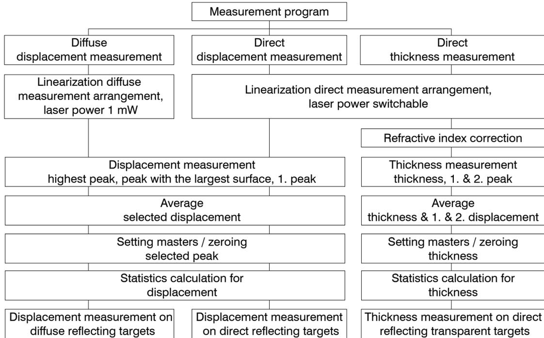
Fig. 31 Adjustment possibilities of the optoNCDT 2300
