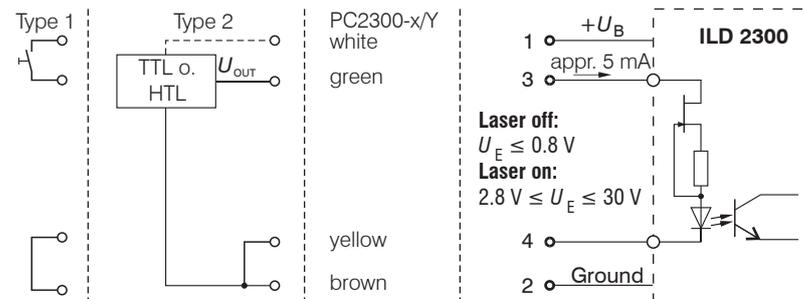
There is no external resistor for current limiting required. Connect Pin 1 with 3 and Pin 2 with 4 for permanent „Laser on“.
