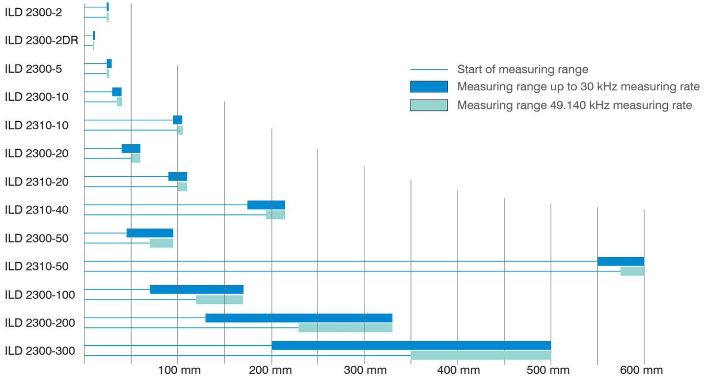
Fig. 7 Measuring ranges for displacement measurement in direct and diffuse reflection
