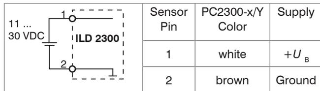
Use the supply voltage for measurement instruments only and not for drive units or similar sources of pulse interference at the same time. MICRO-EPSILON recommends using an optional available power supply unit PS2020 for the sensor.
