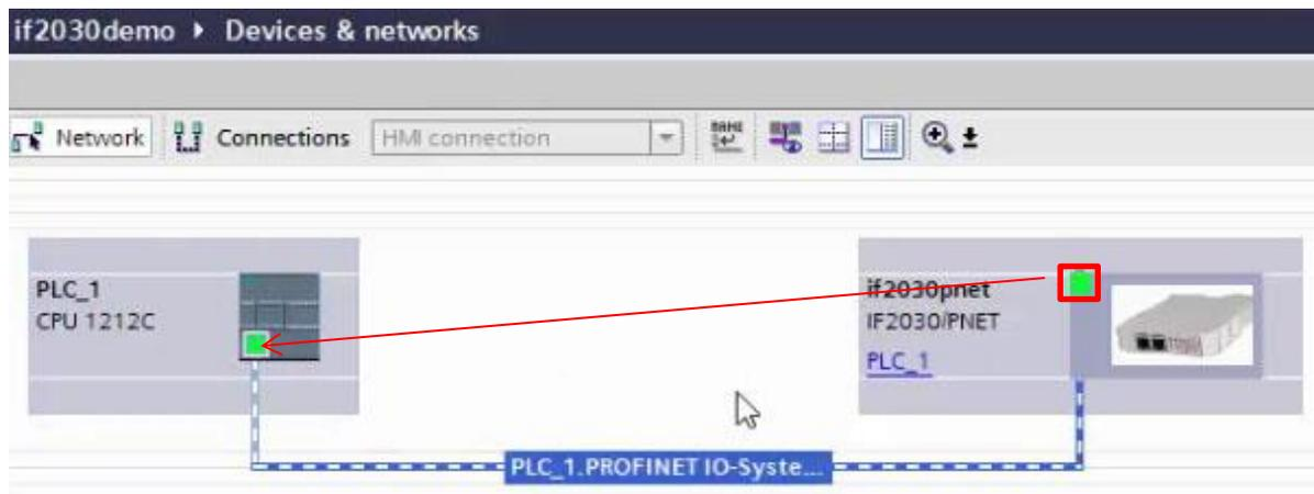
12. Switch to **Device** view, double-click your IF2030/PNET and assign a (device) Name in the **Inspector** window (tab **Properties** → **General**). This name is used for identification in the PROFINET network and as address. Therefore, it must be unique throughout the system!
