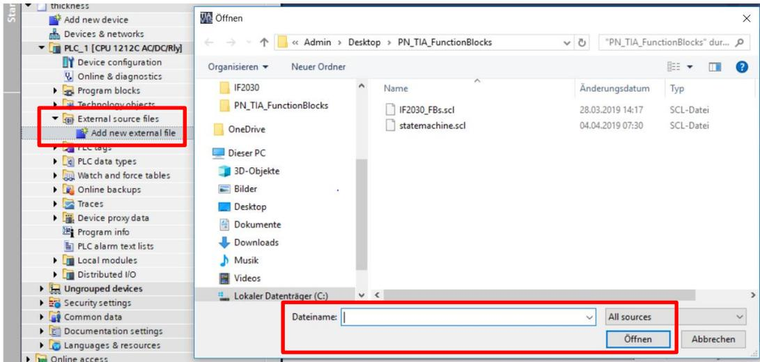
3. When stored correctly, your source file is available in the External source files folder (Project tree). Now transfer the function blocks from the source file to the Program blocks folder. Therefore, right-click the source file to open the Shortcut menu and select the Generate blocks from source command. Confirm the message which may appear informing that existing blocks will be overwritten.
