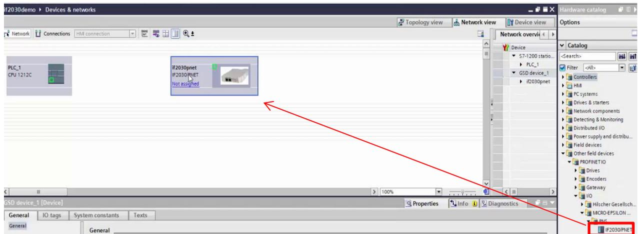
11. Connect the green Ethernet socket of IF2030/PNET with the one of the PLC by clicking one of the green boxes with the left mouse button. Hold the button and draw the resulting line to the other green box in order to create a PROFINET subsystem.
