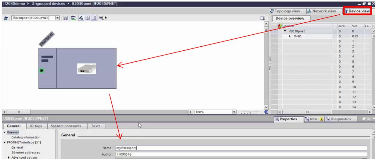
13. The change of name has to be communicated to the PROFINET network. Right-click IF2030/PNET to reach the function Assign device name in the displayed Shortcut menu.
