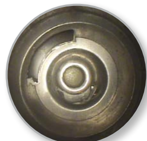
Checking brake cylinder for burrs
