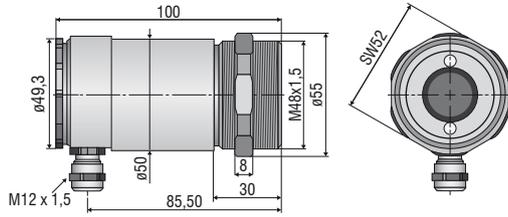
**CS****Sensor mit integriertem Controller****CF Vorsatzlinse (optional)**
