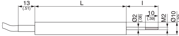
Fig. 7 Displacement sensor type - CA with integral cable, dimensions in mm (inches), not to scale
