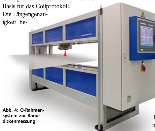
Fig. 4: O-shaped frame system for measuring sheet thickness
